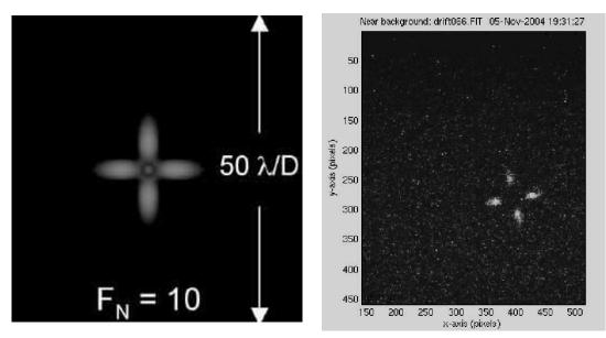
Above left is a computer simulation of a star behind an occulter compared with actual ground test data of Polaris (above right) taken on November 5, 2004. The diffraction lobes are distinctly visible in the computer simulation and in the image of Polaris.
