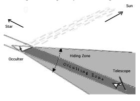
mission designed to perform extrasolar planet detection, orbit determination, and atmospheric characterization about 50-100 or more stars within 15-40 parsecs could be conducted in concert with JWST. Simulations show that a 6.5-m telescope and a 45-m occulter at 20,000 km could detect terrestrial planets in the near-IR about stars out to ~5 parsecs. Moving the occulter to larger distances from the telescope increases the stellar distance for planet detection.
