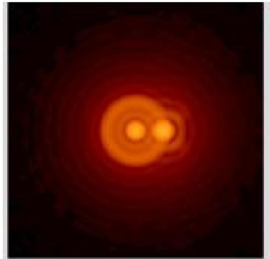
**Figure 5 – Star leakage and Planet at the IWA. Star leakage appears like spherically aberrated halo due to ripples within the aperture.**
