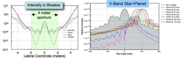
**Figure 3** – Left: Relative intensity in the shadow (at telescope aperture) for monochromatic, V-band, Open (0.4 – 1  $\mu$ m) and a water band. Right: Planet crossing the edge of the occulter as shown in the focal plane.
