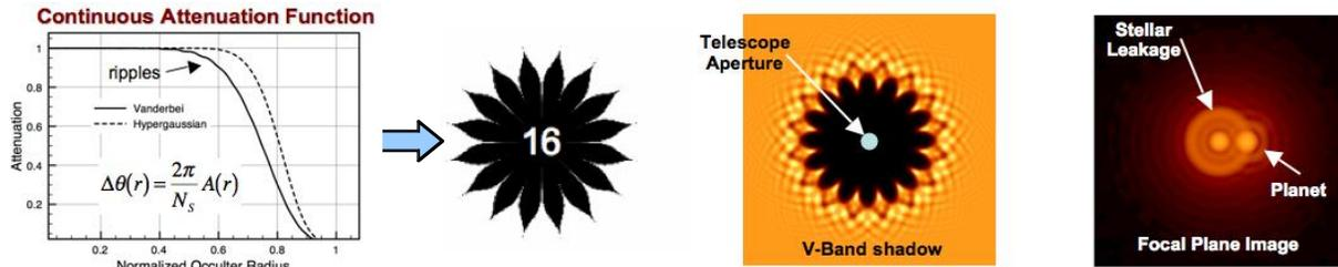
**Figure 2** – Left: Vanderbei and Hypergaussian apodization functions yields a binary 16 petaled mask with approximately the same intensity in the center of the shadow (2<sup>nd</sup> panel from right). Right: Occulted Coronagraph image of a planet and star leakage.
