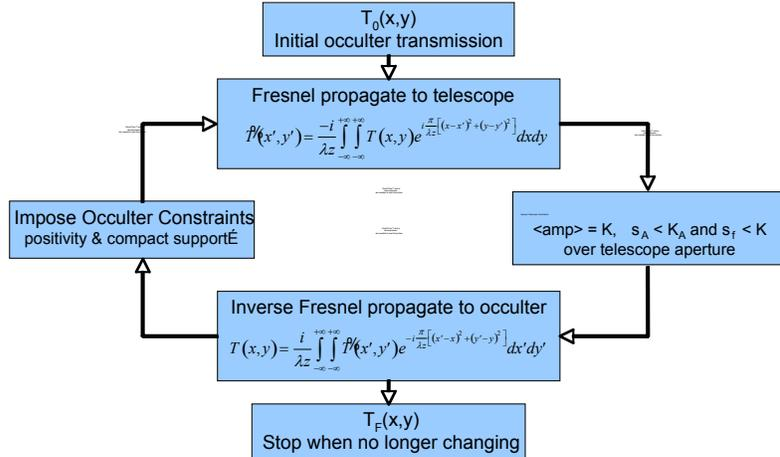
Figure 6 – Iterative Fresnel propagation Algorithm
