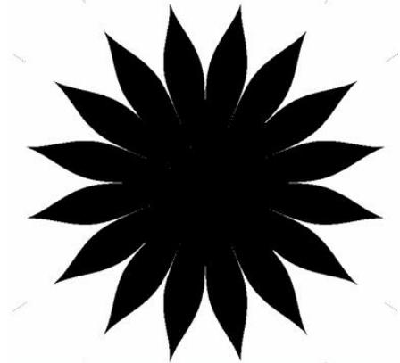
**Figure 8** – Occulting mask designed from Iterative Fresnel Algorithm. There are small ripples along the inner edge of the occulter near the central blocking region.
