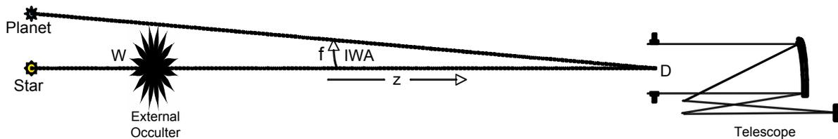
Figure 1 – Externally Occulted Coronagraph Principle
