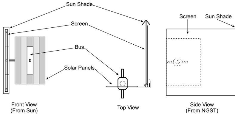
**Figure 4.** SPIDER overview. The four main structures are the occulting Screen, the Sun Shade, the spacecraft Bus, and the Solar Panels.
