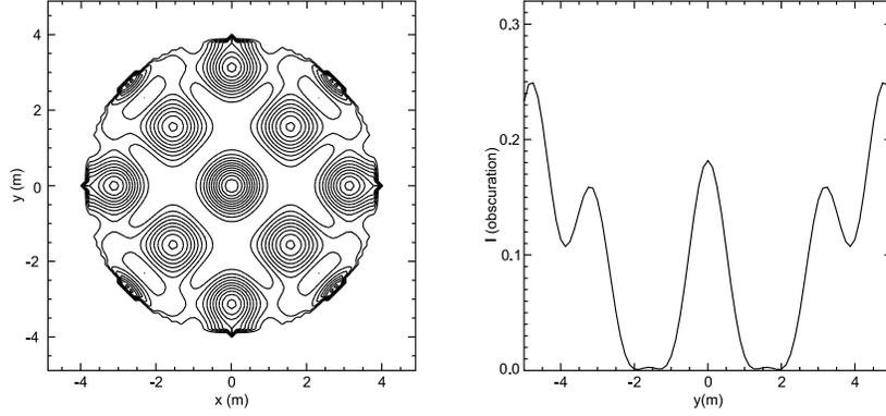
**Figure 3.** The contour map (left) of the Fresnel diffraction pattern covers an 8-m diameter circle in the shadow of a 16-m occulter. The region outside the circle is not of interest and has been eliminated from the figure. The intensity profile (right) is down the center of the diffraction pattern including regions outside the 8-m diameter circle.
